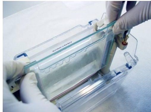
Figure 9. Insert the glass sandwich into the electrode module. Slide the sandwich closely along the pink silicone rubber on the middle part of the module making sure the inside of the gel sandwich risers.
