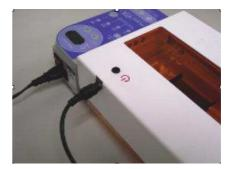
**Step 6:** Push the ON/OFF button of the SmartViewer for real-time fluorescence observation
