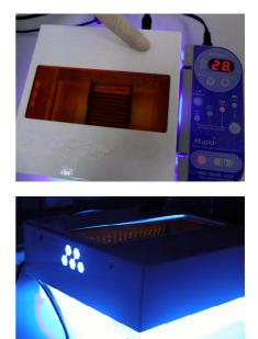
Solution Continuous or frequent LED lighting during electrophoresis of gels may decay the DNA fluorescence intensity.
